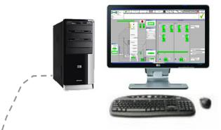
Start-up of the dryer is done in only 3 steps. First start Fans then Burner and when temperature is right then start the Discharge.
