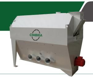
The drum scalper is intended for separation of coarse impurities such as straws, strings, paper, splinters of wood, maize husks etc. from granular or mealy bulk products. Elimination of these impurities will exert a favorable effect on the functional reliability and performance of the machines and conveying elements of the processing line.
